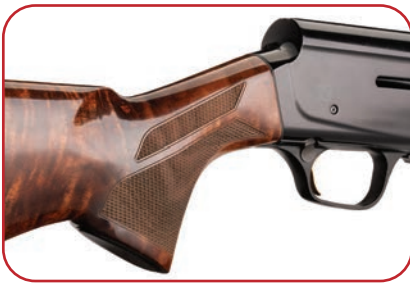
Cut checkering (18 l.p.i.) on the fore-end and the stock's wrist both looks good and aids in control of the gun under recoil.
