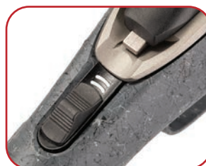
The tang-mounted safety has three positions (l. to r.): "fire," indicated by a red arc; "safe," which blocks the trigger but allows the bolt to be racked; and "safe-locked," which blocks both the trigger and the bolt.
